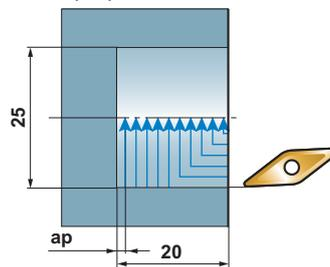
Machining a workpiece with a prepared hole.
