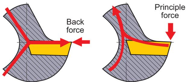
The Dimple bar design effectively balances the principal and back forces, and reduces deflection by up to 17%.
