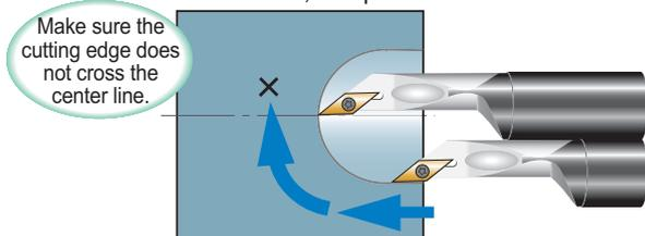
Crossing the center line can chip the insert.
