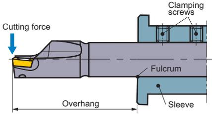
(2) When machining with the holder reversed, the overhang should be measured from the tip to the first clamping screw as shown.
