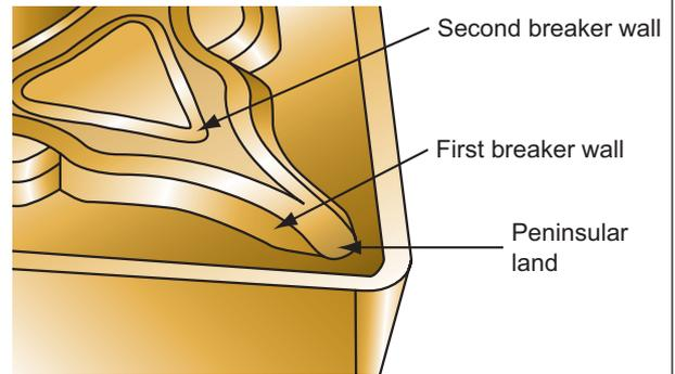
The rake angle ensures sharp cutting to prevent vibrations and gives an excellent surface finish.
