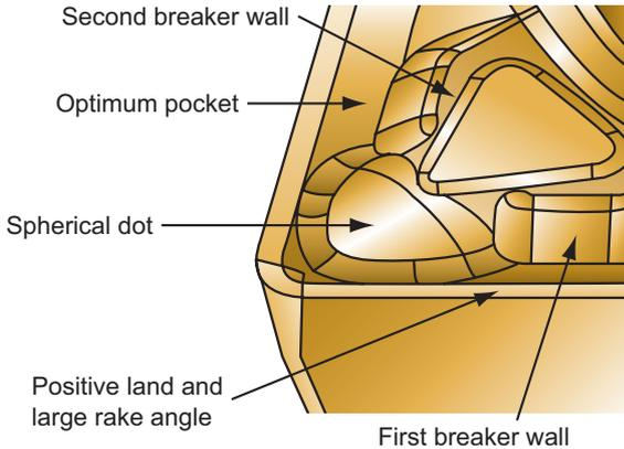
A large rake angle for sharp cutting and longer tool life.
