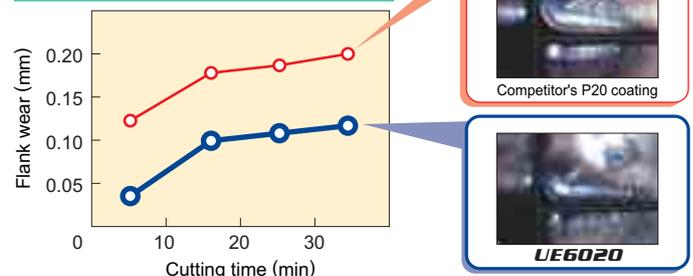
Holder : FSCLP2220L-09E Workpiece : JIS SCM440
