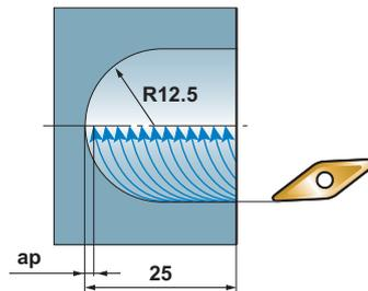
Machining a workpiece with a prepared hole.
