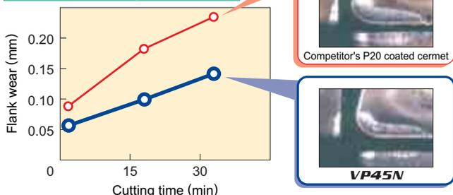
Holder : FSCLP1816L-09S Workpiece : JIS SCM440
