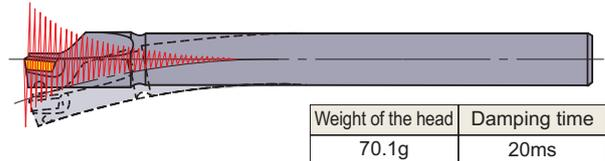
By reducing the weight of the head, the damping properties are increased.
