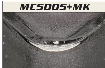
Wear 0.29 mm After machining 30 pcs.
