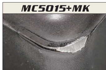
Wear 0.44 mm After machining 17 pcs.
